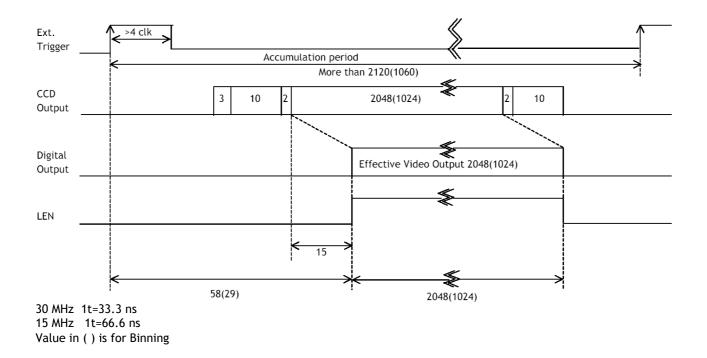
Fig. 14. Timing for external trigger scan mode
